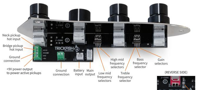
NOTE: Pickup grounds, bridge and/or shielding grounds can be used in any ground connection terminal
