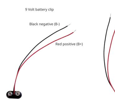
Connect one red (+) wire from one battry clip to the black (-) wire from the other battery clip for **18 volt operation**.
