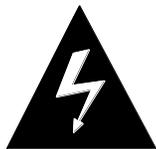
The lightning flash with arrowhead symbol within an equilateral triangle is intended to alert the user to the presence of uninsulated dangerous voltage within the product's enclosure that may be of sufficient magnitude to constitute a risk of electric shock to persons.
