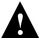
The exclamation point within an equilateral triangle is intended to alert the user to the presence of important operating and maintenance (servicing) in the literature accompanying this device.
